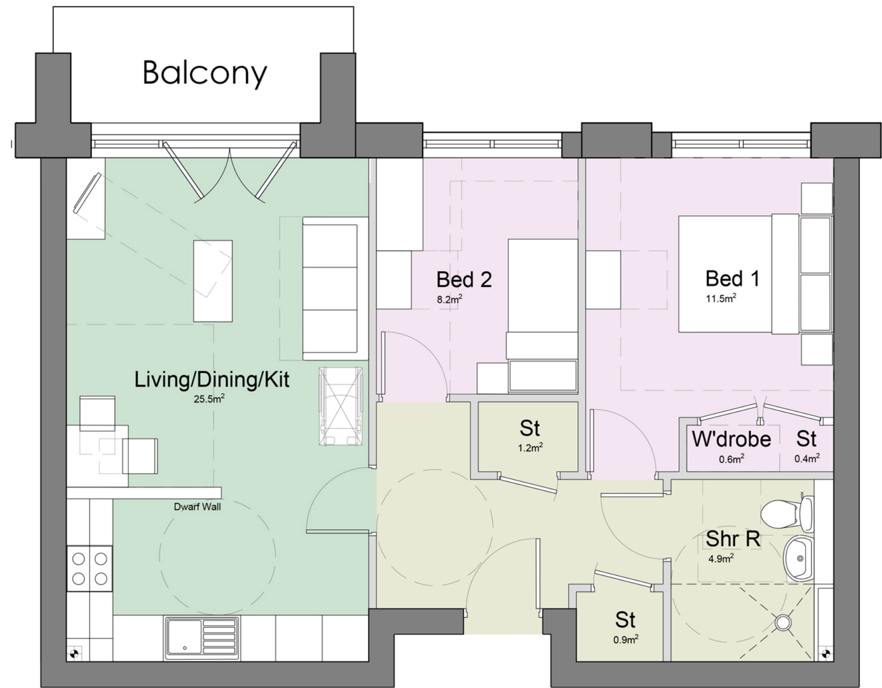
2 Bed 3 Person Apartment - 62.5 sqm NDSS Min Area - 61 sqm NDSS Min Storage - 2.0 sqm NDSS Min Double Bed Area & Width - 11.5 sqm / 2.75m NDSS Min Single Bed Area & Width - 7.5 sqm / 2.15m
